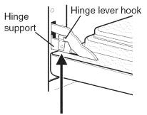
Lock engaged for door removal Figure 1
